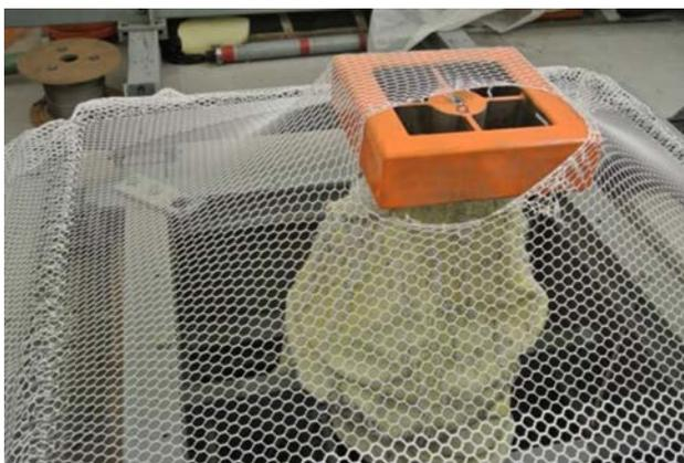
Figure 2: Determination of the main breaking force [STFI e.V.]
