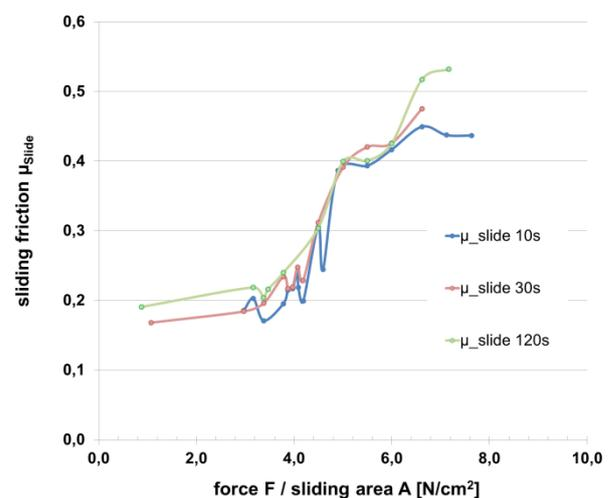
Figure 5: Sliding behavior of anti-skit system after different resting times
