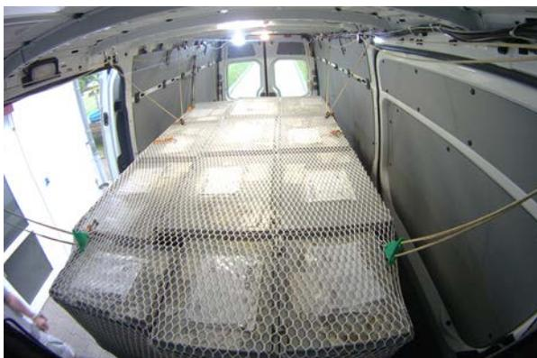
Figure 11: Cargo hold with load securing system
