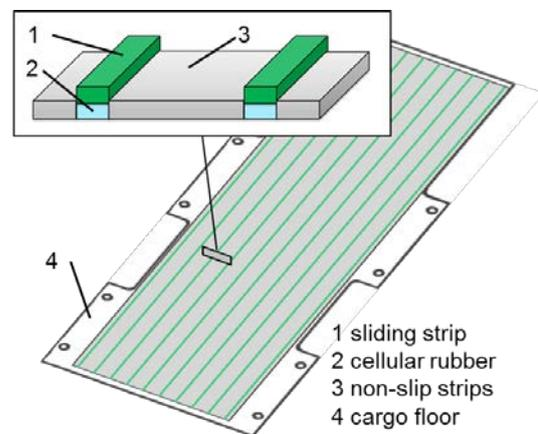
Figure 4: Structural composition of anti-skit system
