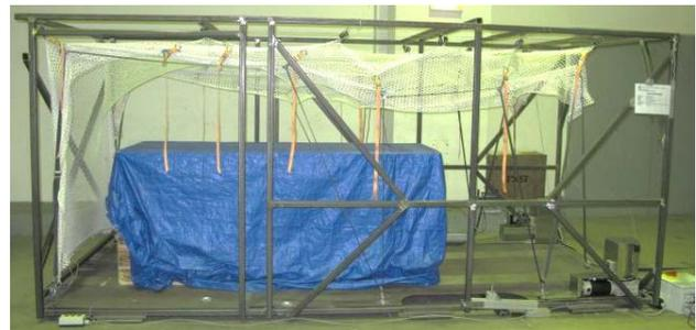
Figure 8: Left side, open net, cargo height 1.0 m
