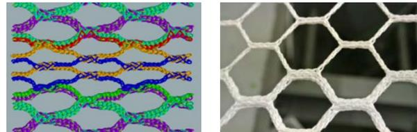
Figure 3: Computer-aided mesh construction (l.), Passage single/double net mesh legs (r.) [STFI e.V.]
