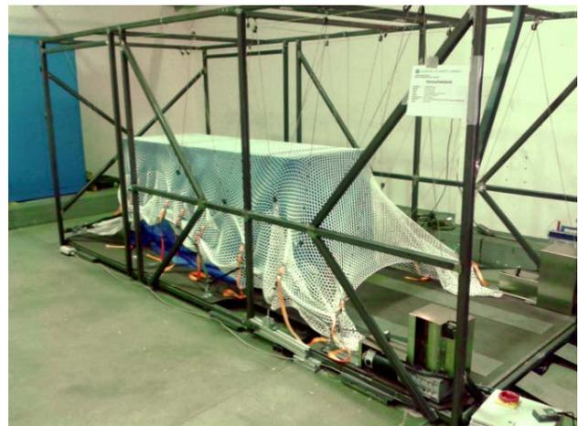
Figure 9: Left side, lashed net, cargo height 1.0 m
