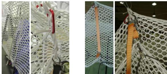
Figure 6: Shortener – advancement of Isilink<sup>®</sup> with high-strength filaments for 3d transmission of force (l.), clamping lock straps (r.)
