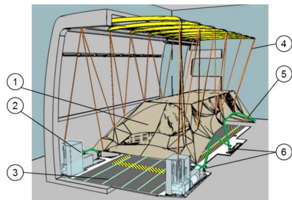
Figure 1: Automatic load securing system in lashed position
