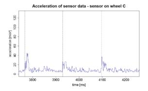
Figure 4.: Acceleration of sensor data over 3 wheel rotations Sensor on wheel C
