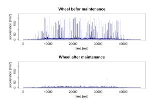
Figure 7.: Reference run of an ASRS a) before maintenance b) after maintenance
