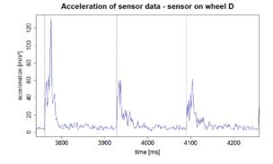
Figure 5.: Acceleration of the sensor data over 3 wheel rotations Sensor on the wheel D
