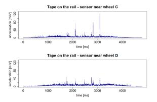
Figure 6.: Sensor data tape on rail a) Wheel C b) Wheel D
