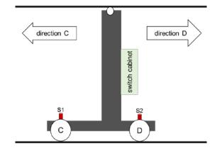
Figure 1.: Schematic structure of an ASRS and placement of the sensors
