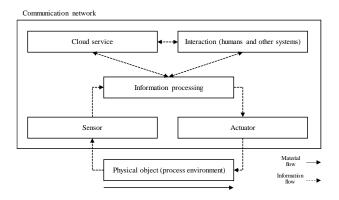
Figure 2. Dependencies of the technical components of a CPS
